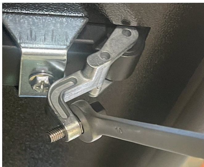
10mm spanner on locking nut
