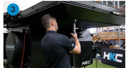
3 Secure the two support poles.
