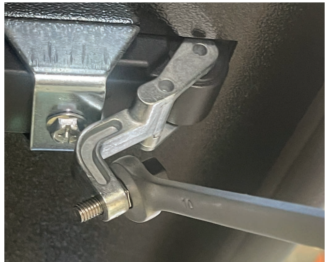
10mm spanner on locking nut
