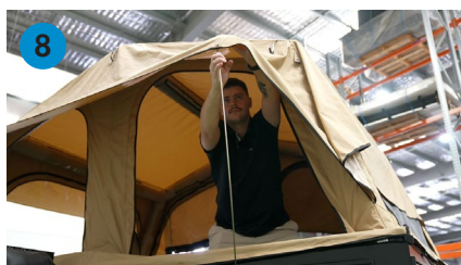
Attach the included poles to support the window rain flaps.
